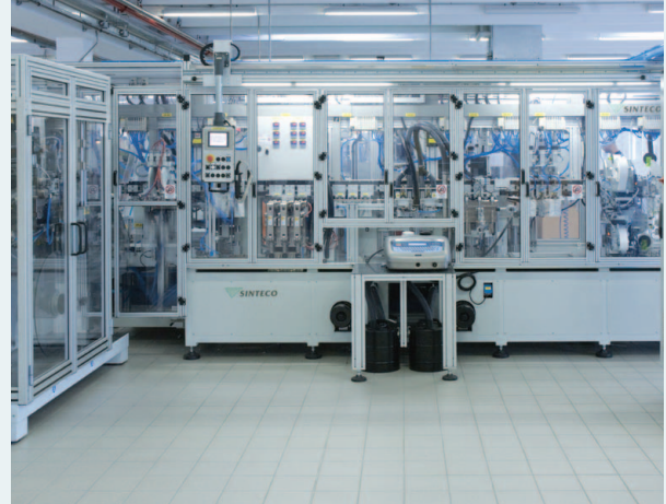
Below, a view of the Coster 3 and Coster 4 plants located in Caldonazzo, Italy. Coster 3, to the right in the photograph, is one of the most advanced and highly automated plants in the aerosol valve sector. Automation is governed by an integrated, computerized system that continuously monitors the entire production flow, from the dosage of the raw materials in the silos to the moulding, collection of moulded components by laser-guided robots, sorting and finally packaging and preparation for shipping. Also manufactured in Coster 3 are the valves used in the Coster 4 facility, dedicated exclusively to the production of Bag-On-Valves. Left, Coster USA, Inc., South Elgin, Illinois: the factory is located near Chicago's O'Hare Airport. Assembly of 1" valves and bag placement are performed at this facility.
